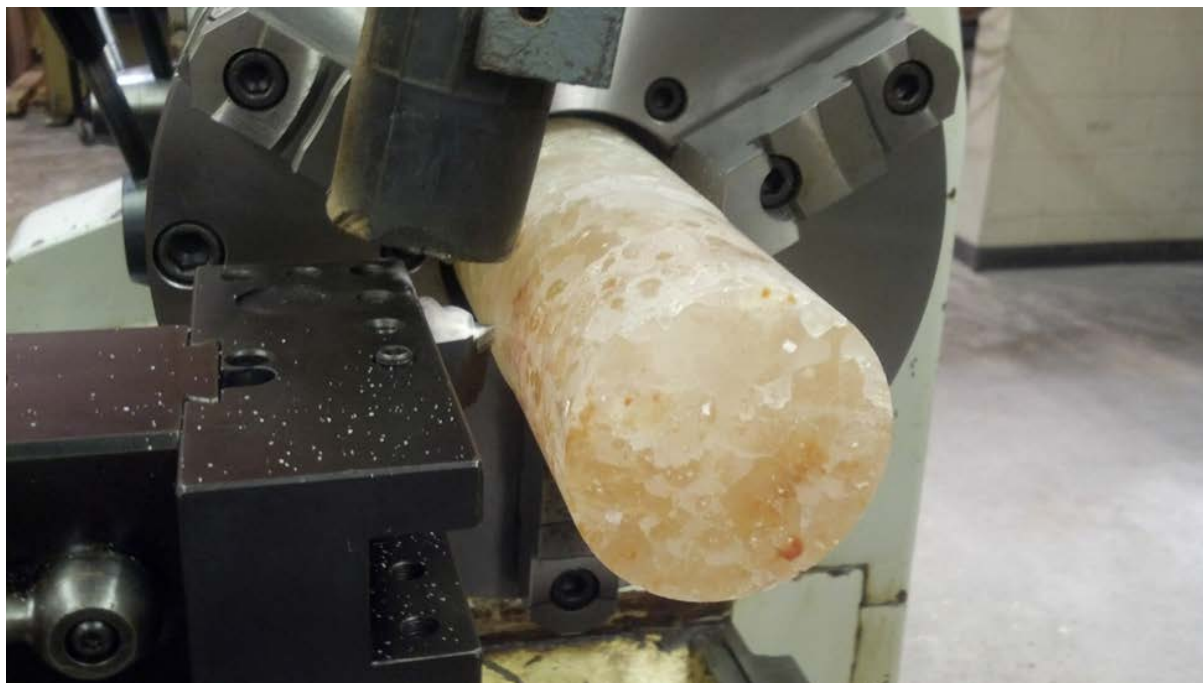
Figure 1. Typical Machining Setup for Preparing Cylindrical Specimens.
