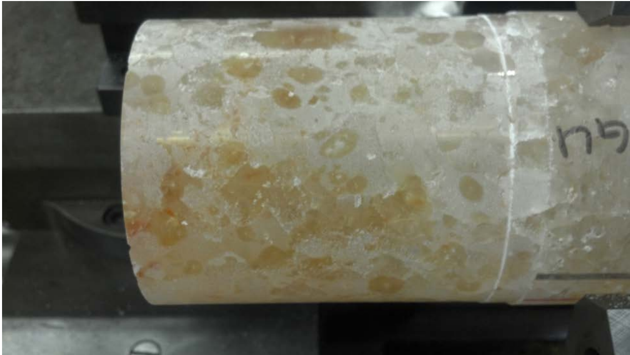
Figure 2. Bedded Salt Specimen Brine Inclusions (darker ovoid areas are wet).
