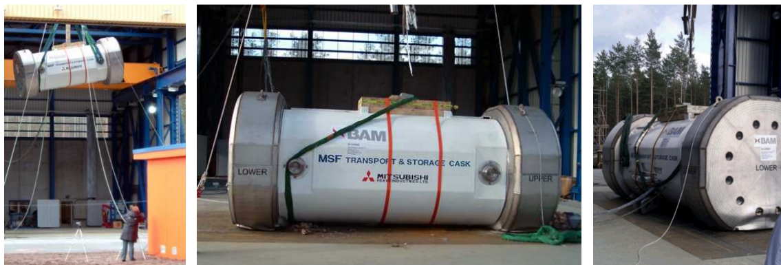
Figure 1-5 BAM MHI-MSF69 BG shallow angle drop test (BAM public website).
