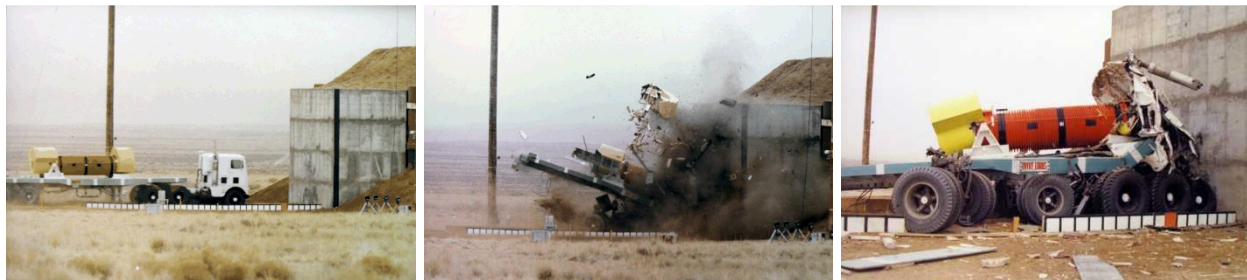
Figure 1-6 SNL truck cask demonstration test at 130 km/h (80 mph) (Jefferson 1978).
