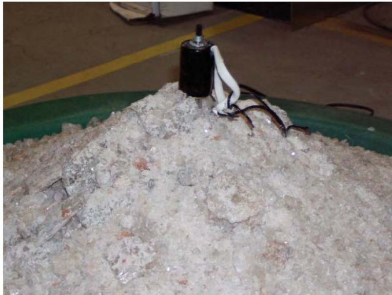
Figure 3-11. View of the experimental set-up corresponding to the thermal test on a pile of crushed salt (Stauffer et al., 2013).
