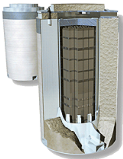
Figure 1.1 Typical vertical aboveground storage cask system.
