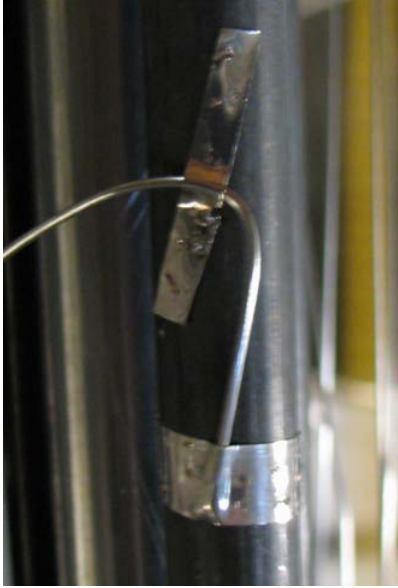
Figure 2.5 Typical TC attachment to heater rod.
