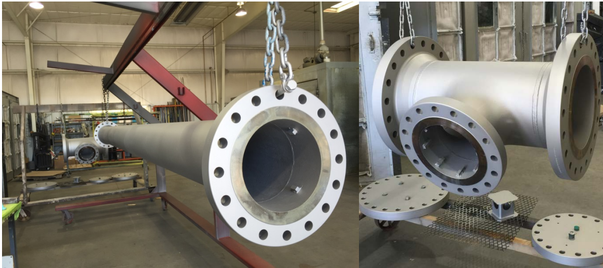
Figure 4.1 Carbon steel pressure vessel components freshly coated with high temperature paint.
