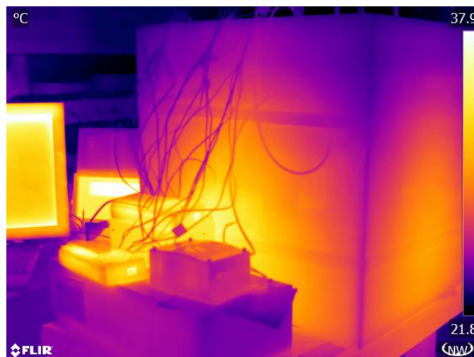
Figure 28: Infrared imaging of salt box at maximum temperature of 260 °C.
