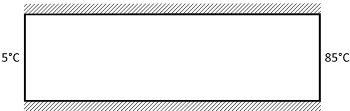
Figure 12: Model domain for case with no insulating layers.
