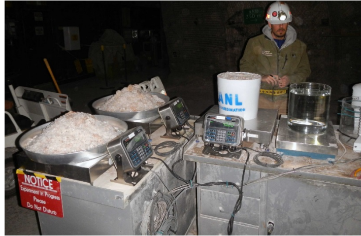
Figure 22: Salt pan experiment in WIPP salt gallery. Pans with salt piles are on left.
