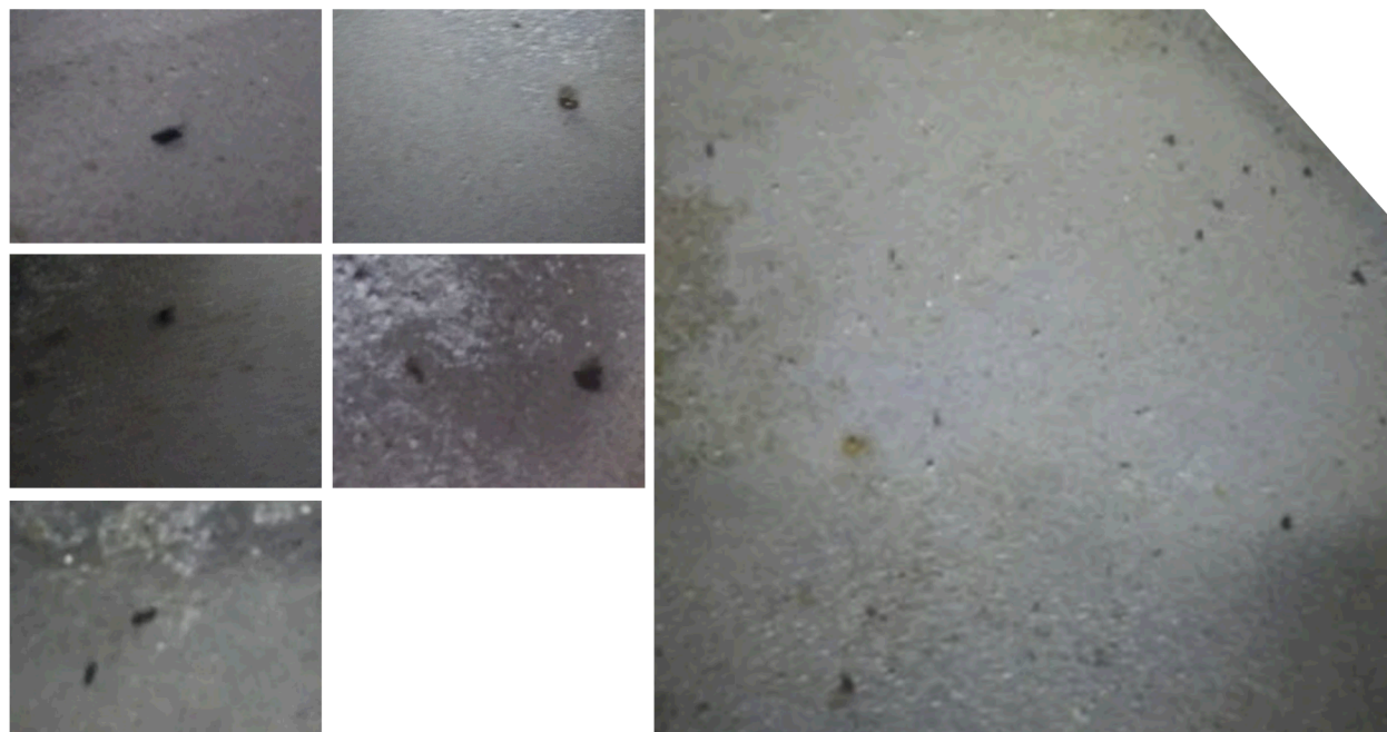
Figure 40. Boroscope camera images of insects on the floor of the HBU storage cask. The scale is not provided in the images, but comparison with structural features in the images (not shown), indicates that the insects are 2-4 mm in size.
