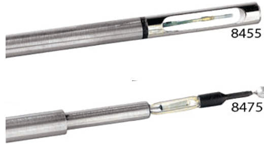
Figure 2.14 Photographs of the two types of hot wire anemometer tips.
