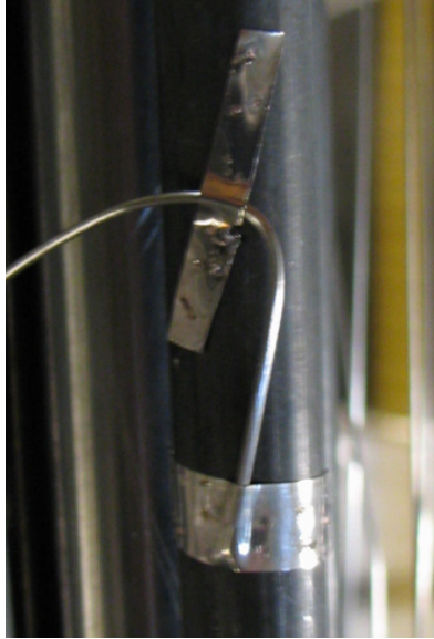
Figure 2.5 Typical TC attachment to heater rod.
