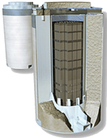
Figure 1.1 Typical vertical aboveground storage cask system.
