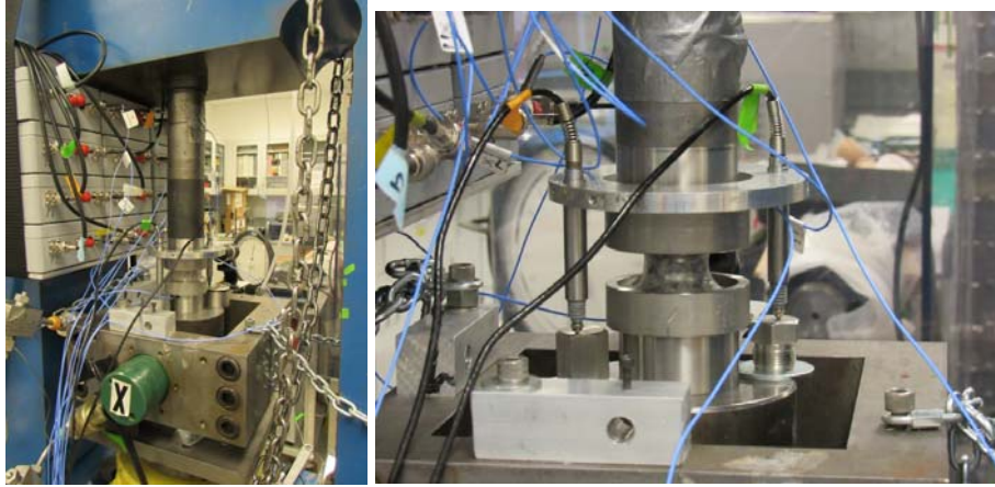
Figure 5-8. Laboratory setup for the shaped-core uniaxial compression experiments using Stripa Granite cores.
