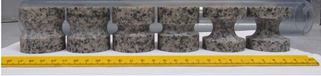
Figure 5-6. Shaped core samples of Stripa Granite. From the left, sample #1 through #6.
