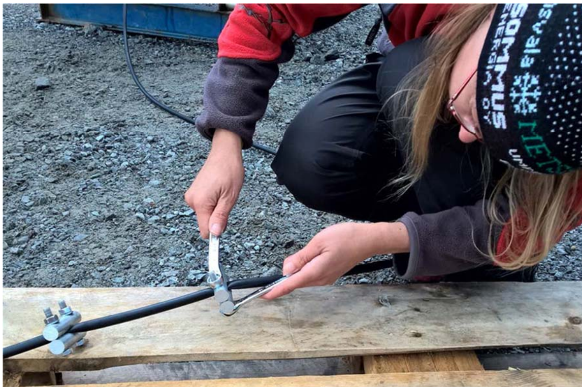
Figure 2-3. Collection of tube samples in the field. Metal clamps were used to crimp the plastic tubing to separate out distinct sampling intervals.
