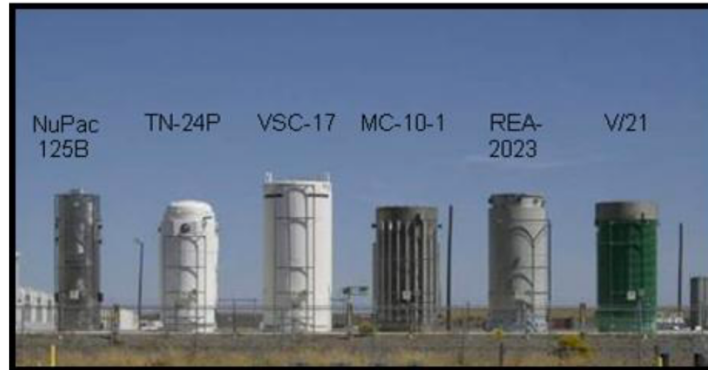
Figure 10. Dry storage casks on the CPP-2707 pad at the INL Site. Note that TN-REG and TN-BRP casks are not pictured.
