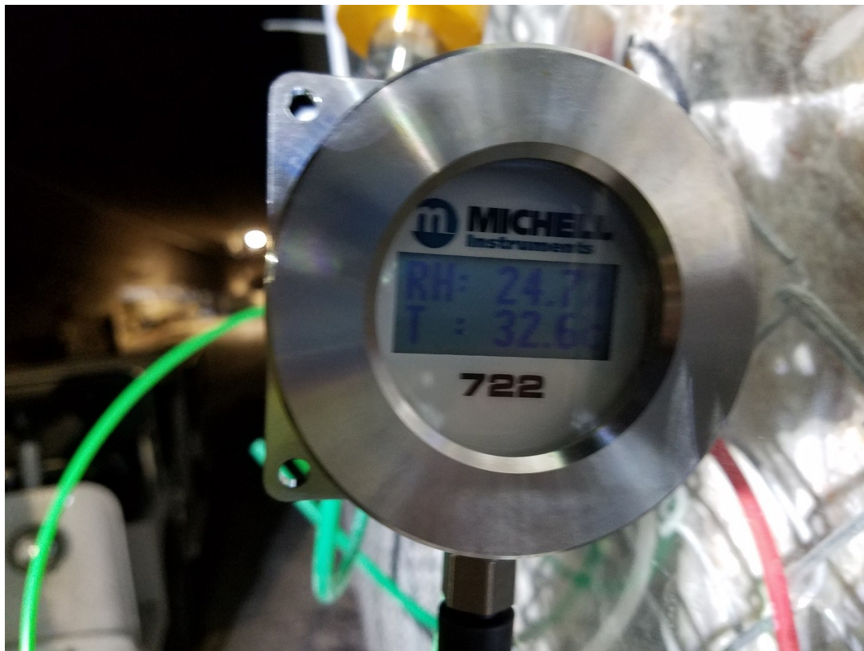
Figure A- 9. Image of the Phase 1 DT722 relative humidity probe used to monitor RH and temperature of the gas circulated in the heated borehole.
