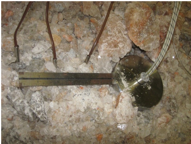
Figure 4. Photograph showing the heater assembly being laboratory tested in Run-of-Mine salt
