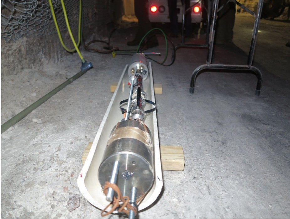
Figure 10. The Phase 1 heater/packer assembly prior to installation.
