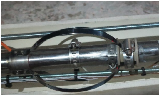
Figure A- 6. Figure showing the LVDT assembly mounted on a 1 in central pipe.
