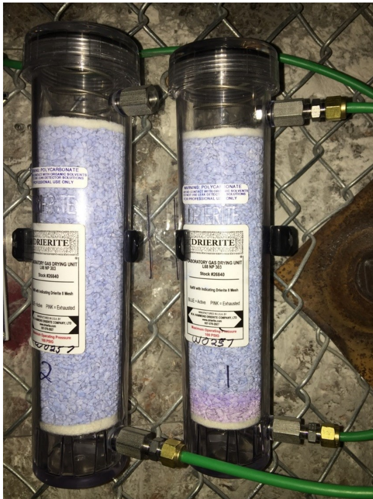
Figure A- 10. DRIERITE cartridges used for Phase 1 moisture capture.
