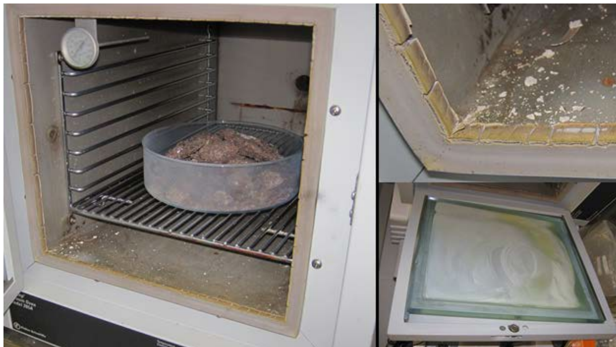
Figure 2-1 Oven Corrosion after Heating WIPP salt from Clay Seam F
