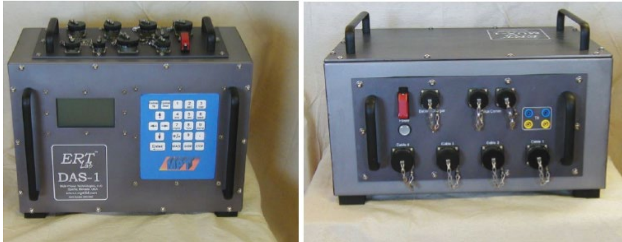
Figure 7-3. Photographs of MPT DAS-1 Electrical Impedance Tomography System that was used for ERT data acquisition.
