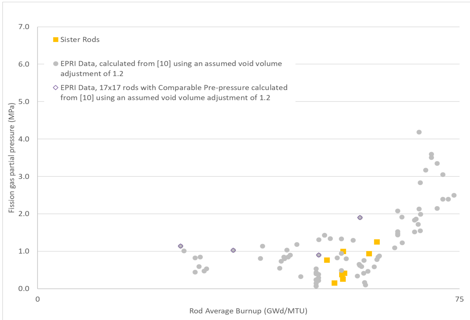
Figure 14. Sister Rod Measured Fission Gas Partial Pressure at 25 °C.
