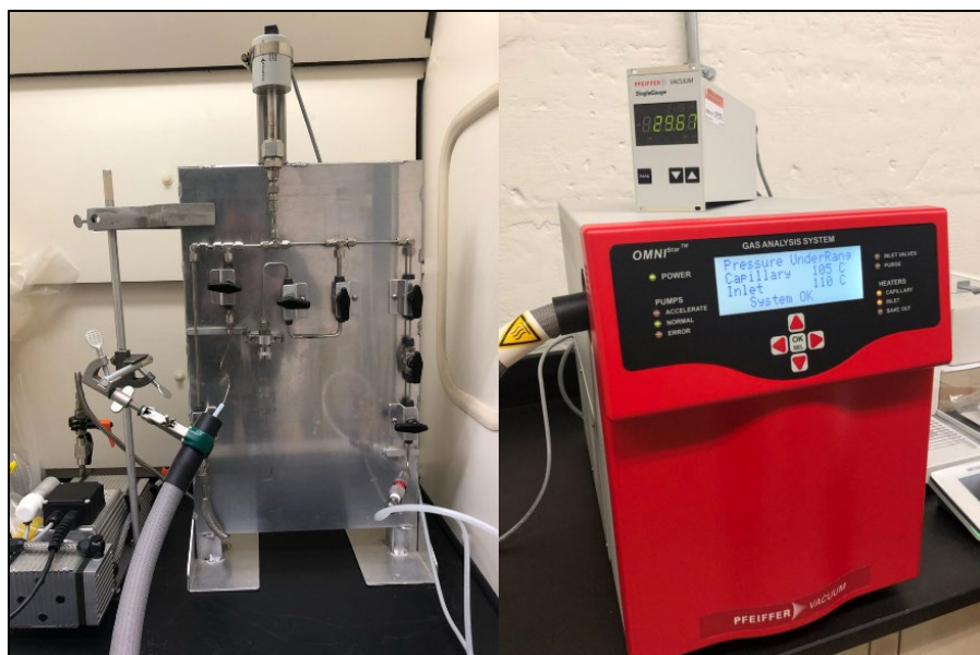
Figure 27. The Sample Inlet Manifold (left) Coupled to an OmniStar GSD 320 Gas Analysis System (RCA) (right).
