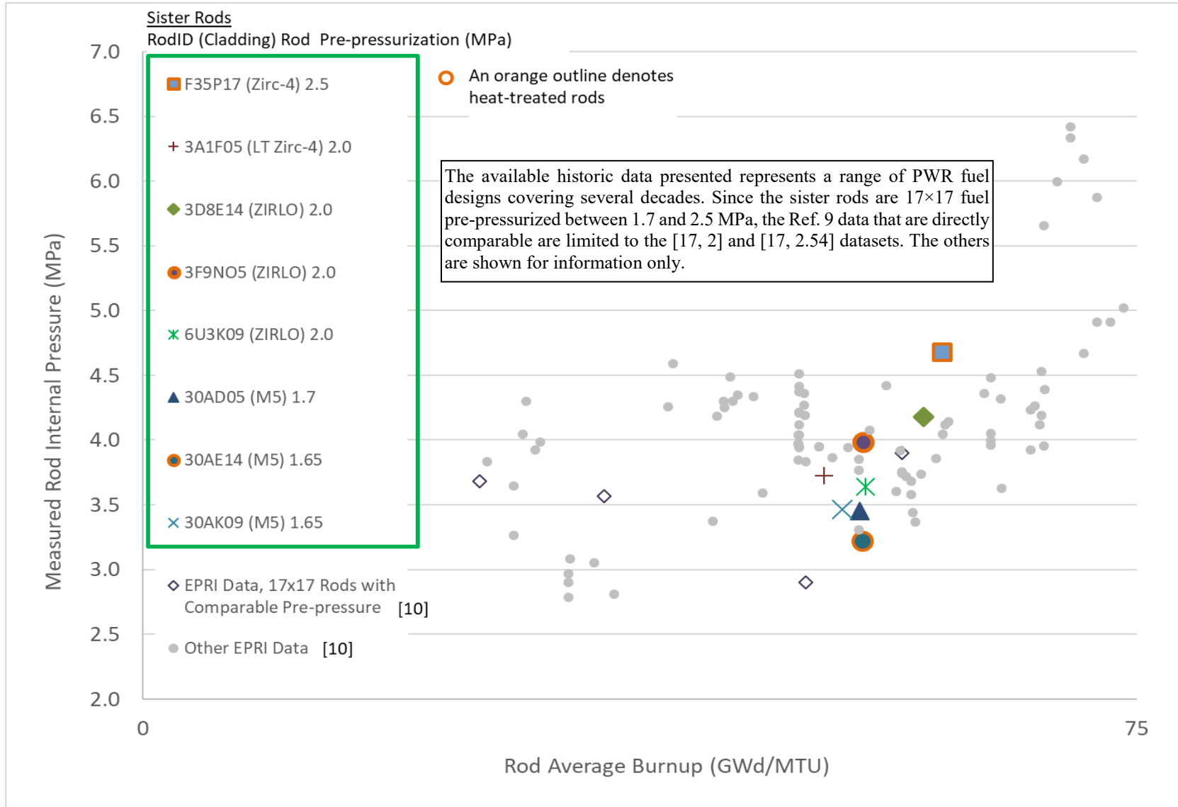
Figure 13. Sister Rod Measured Rod Internal Pressure at 25 °C.
