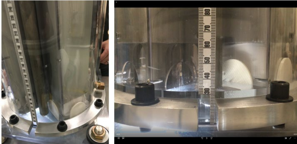
Figure A-18. View of the Blocked Mouse Holes by the Drain Pipe.
