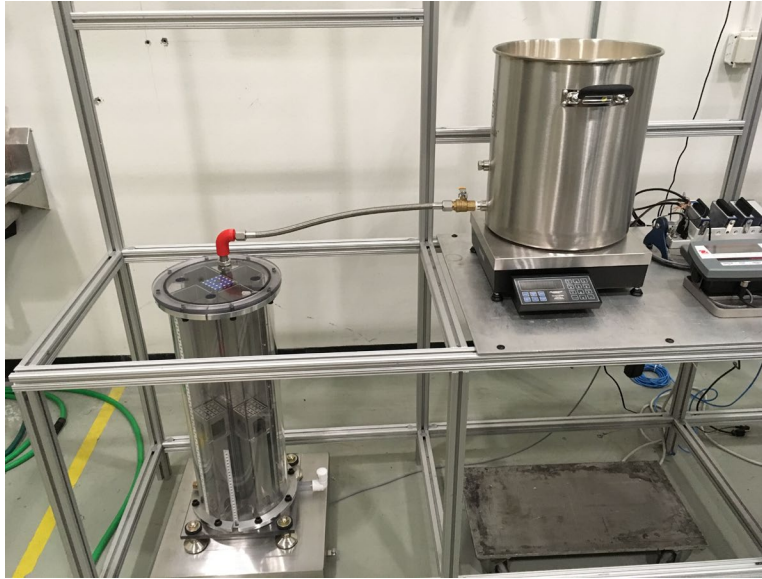
Figure A-23. Glycerin Test System Set Up.
