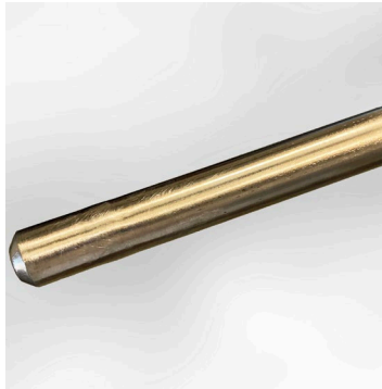
Figure 2.3 View of the welded end plug on the 1000 W heater.
