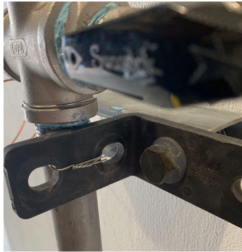
Figure 2.6 Middle cross of pressure vessel tied to fiberglass bracket with Nichrome wire.
