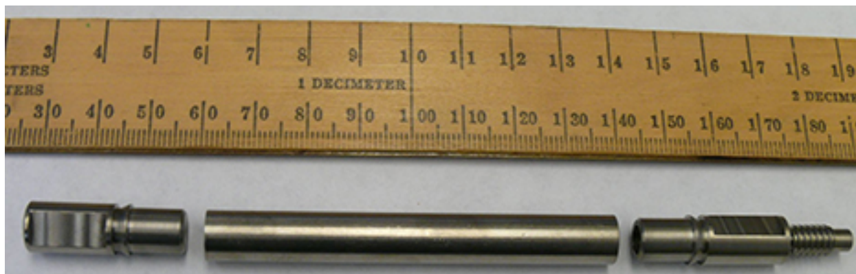
Figure 5: Rodlet bottom end fixture (redesigned), cladding segment, and top end fixture (redesigned).
