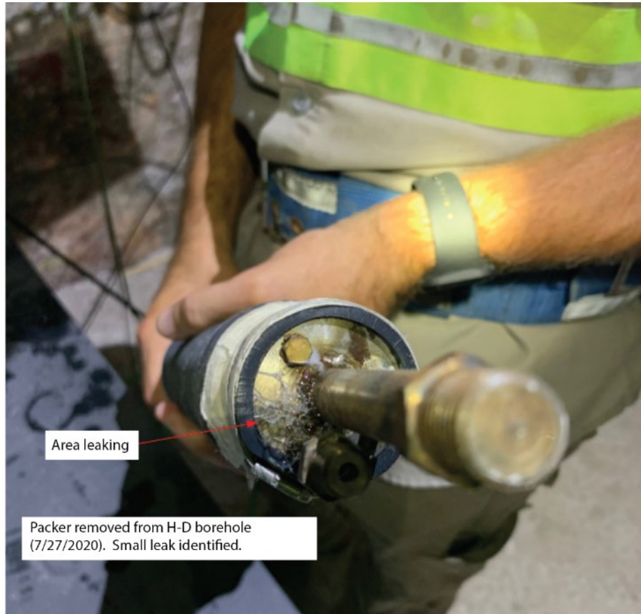
Figure 6-2. Leaky packer detected during permeability experiments.
