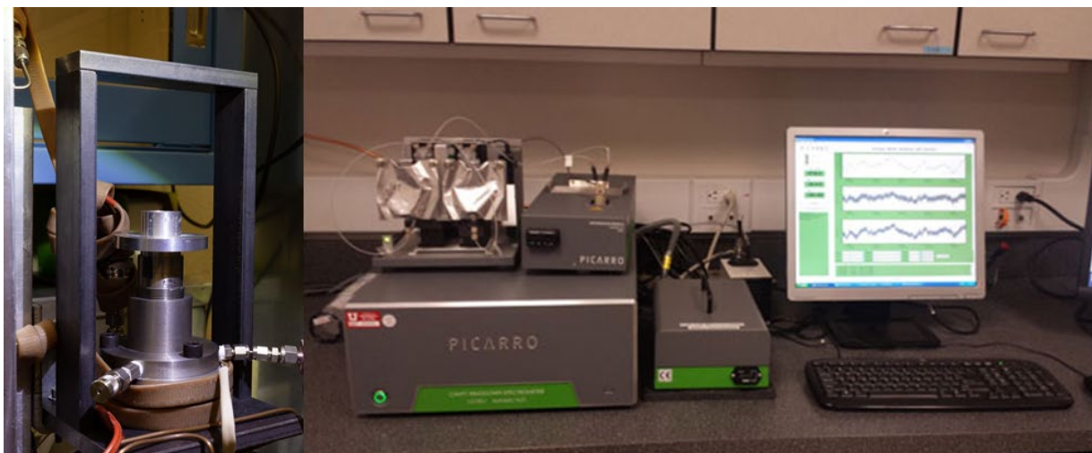
Figure 3-10. Crusher with inlet and injection port on the left. Picarro CRDS on the right.
