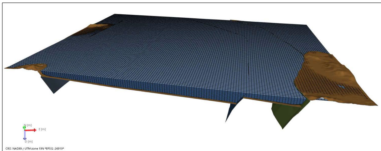
Figure 4-1: The 3D Grid model for alluvial sediments in the Deming sub-basin. Grid cells are 200 m x200 m in the horizontal dimension and 50 m in the vertical dimension.
