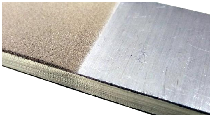
Figure 7. High pressure cold spray (HPCS) coating of commercially pure nickel sprayed at PNNL where the left side of the coupon is cold sprayed and the right side is the base metal.
