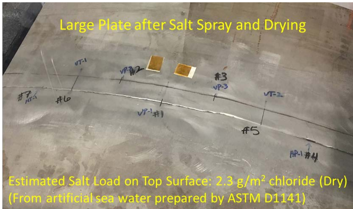
Figure 8. Large plate with EDM starter cracks after salt spray and drying
