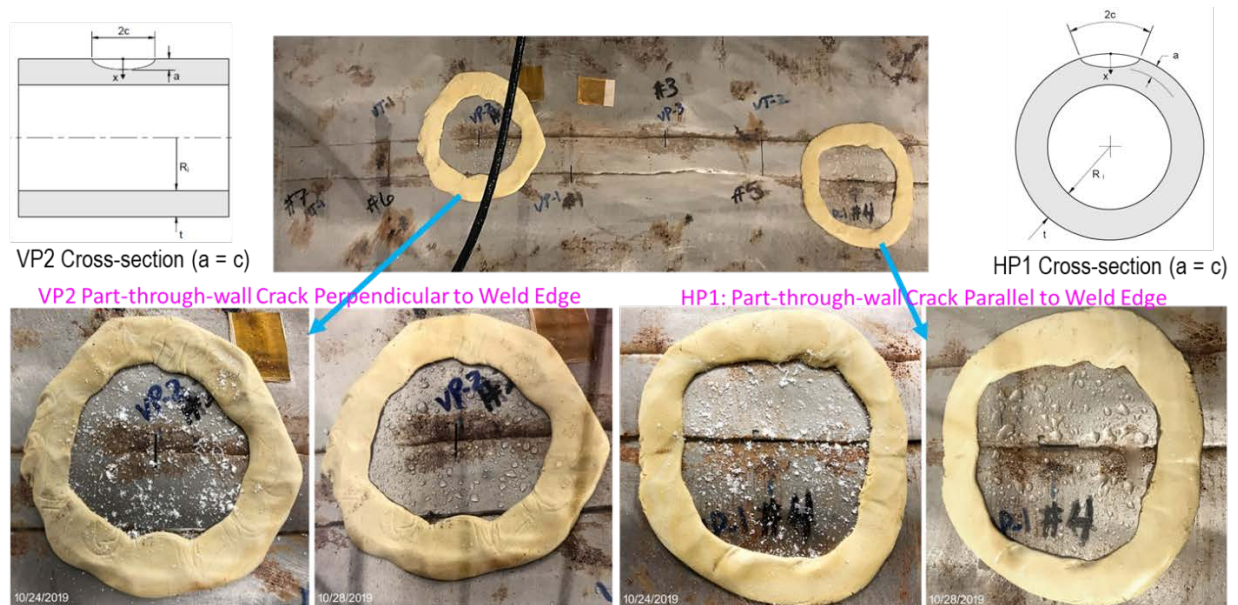
Figure 12. Additional salt applied to selected starter cracks (VP2 and HP1).
