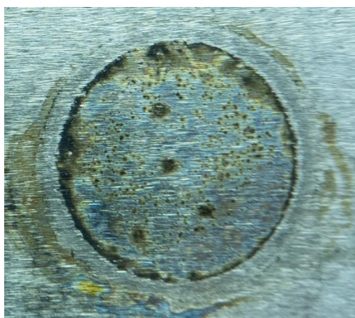
Figure 38. Image of polished C22Gd (1100°C) specimen after PS testing (Figure 37).
