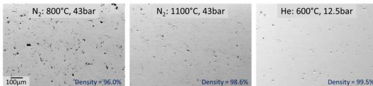
Figure 30. SEM images of the cross-section of C22Gd coatings.
