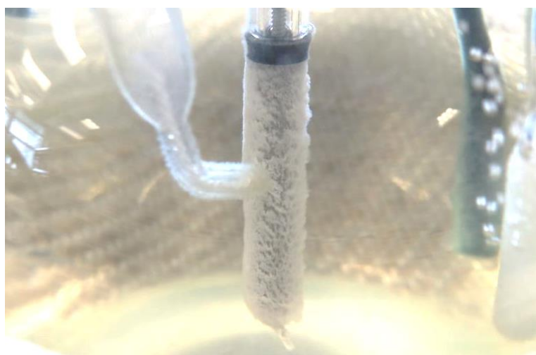
Figure 22. Image of M322 after PS testing before removal from the test vessel showing a significant amount of white corrosion product.
