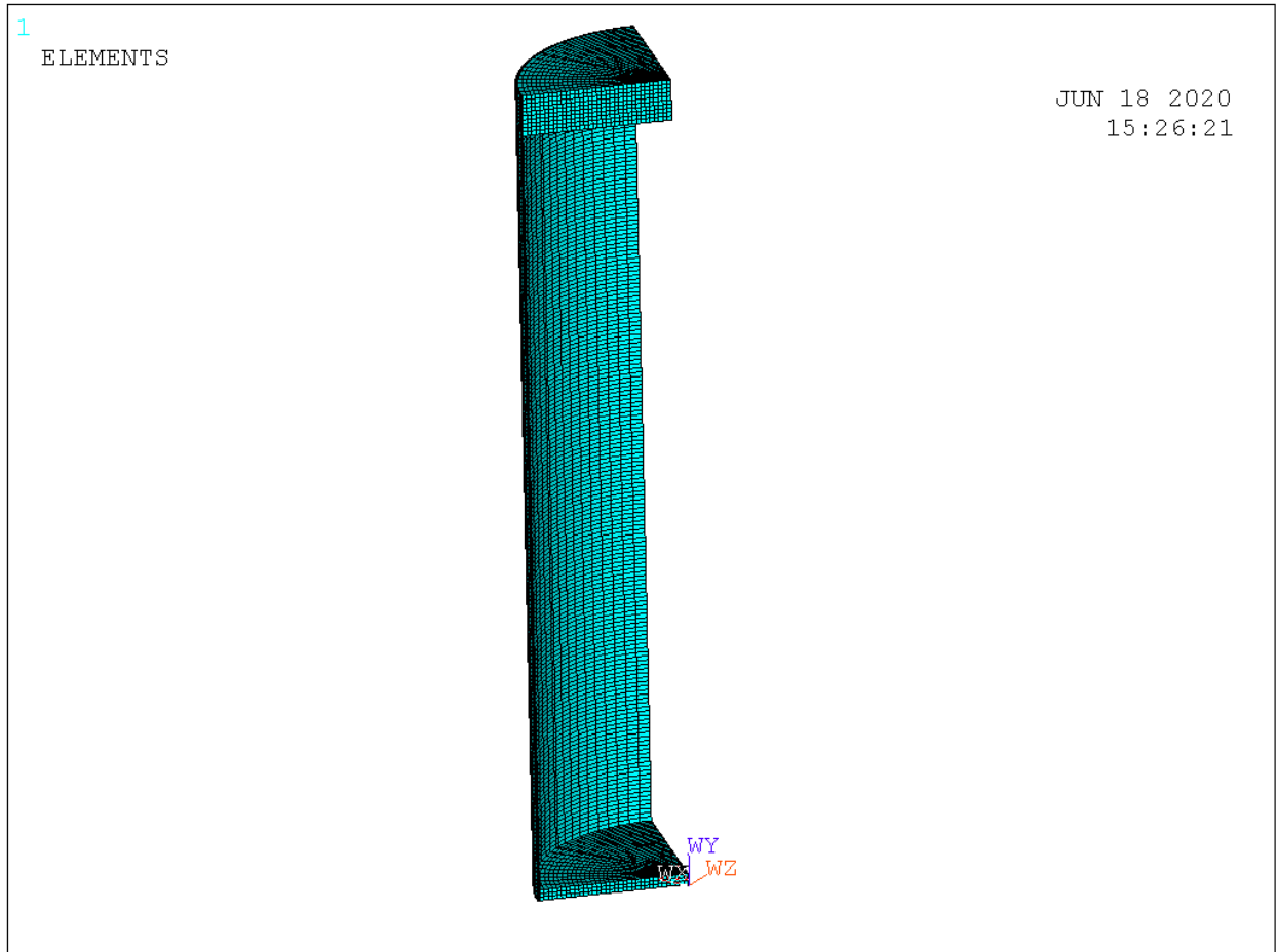
Figure A.4. ANSYS APDL model elements.
