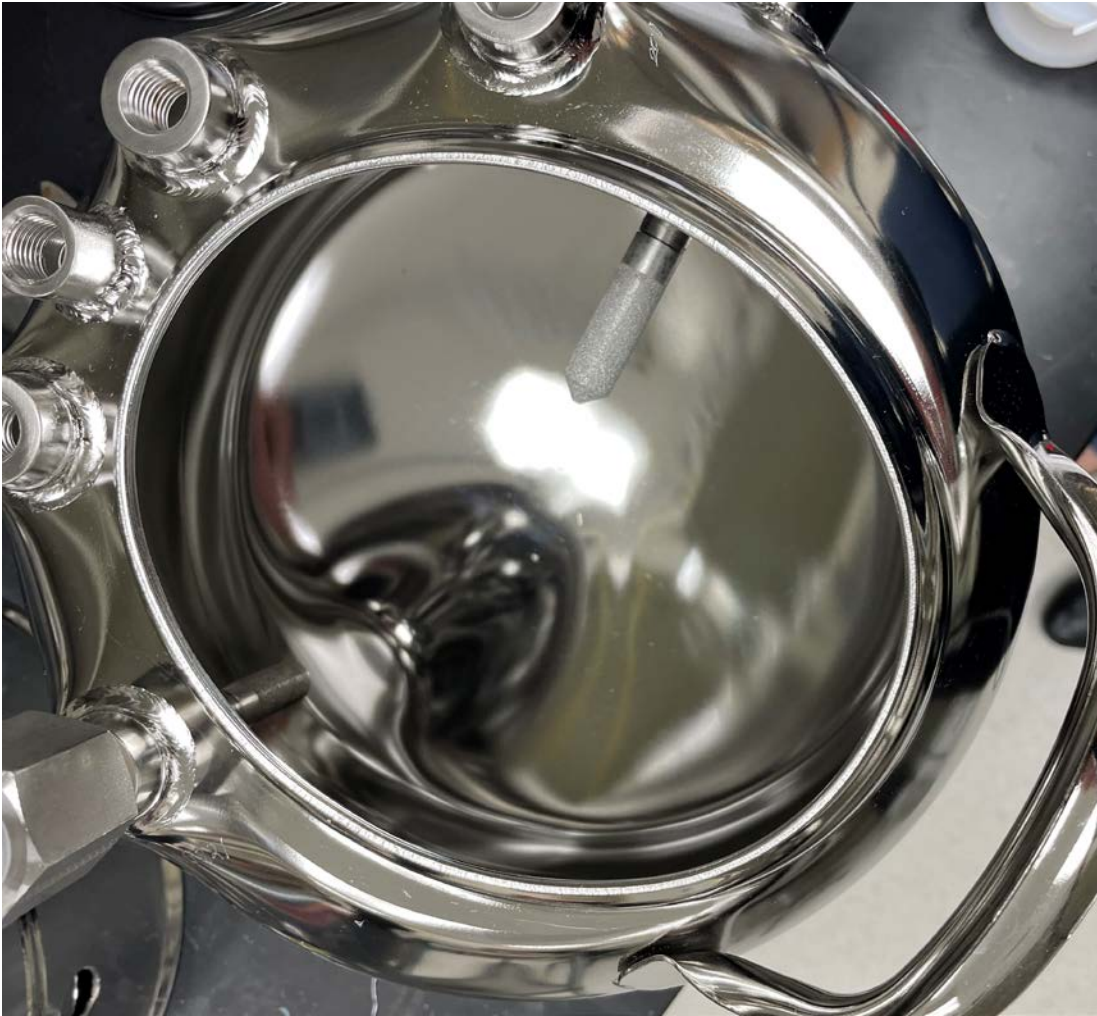
Figure 1. Custom fabricated 1 gallon pressure vessel with two Vaisala HMP4 probes installed.
