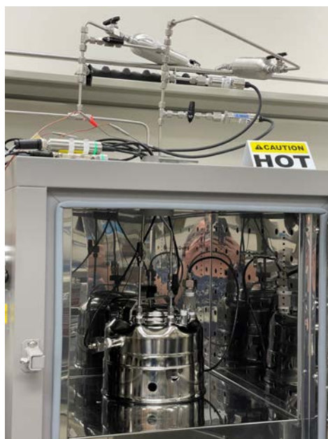
Figure 4. FY2021 Sample bottle configuration testing – VWR oven, two sample bottles in a double-ended configuration this test was repeated with a heated blanket around the upper portion.
