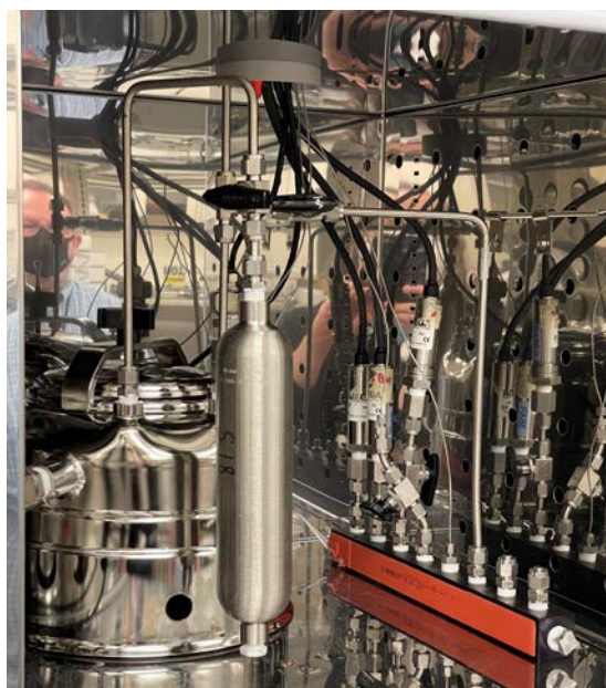
Figure 3. FY2021 Configuration testing, VWR oven, 15” length of tubing between the sample bottle and pressure vessel.
