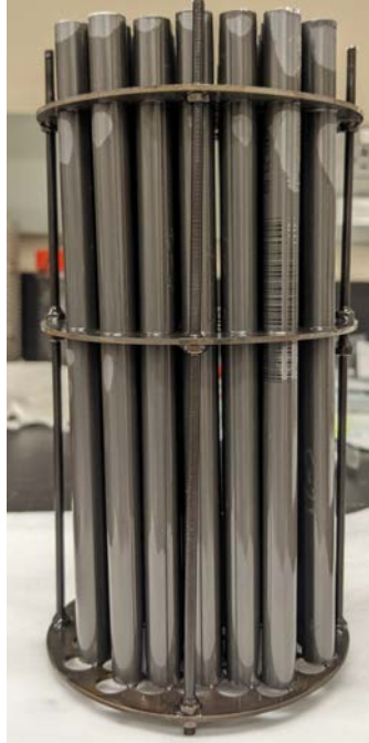
Figure 21. Cladding lengths that have undergone oxidation in the autoclave.
