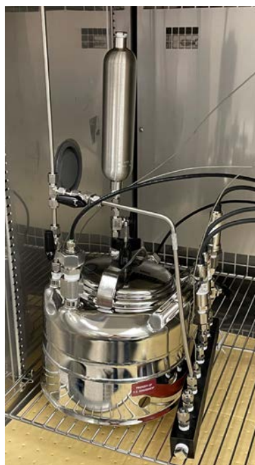
Figure 2. Initial FY2021 bottle sampling configuration test. The sample bottle was connected directly to the pressure vessel to minimize water losses to tubing during expansion.
