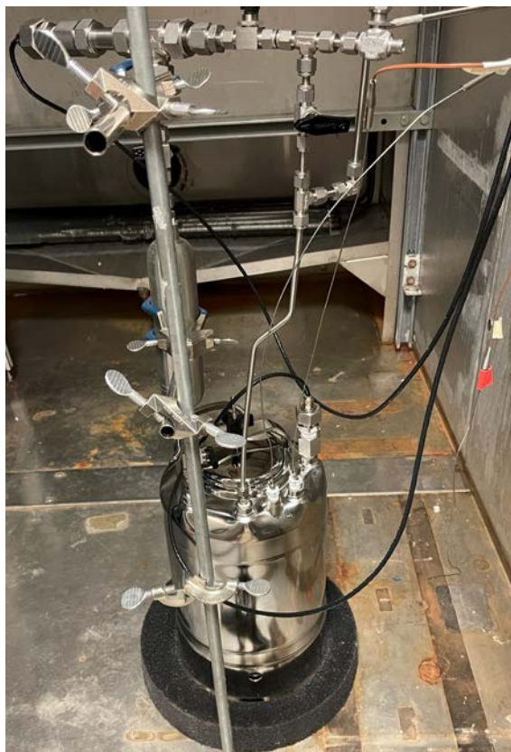
Figure 5. Large environmental chamber with 4-gallon pressure vessel. Second humidity probe mounted horizontally above the outlet of the sample bottle.
