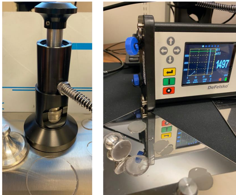
Figure 11. Experimental test of the baseline measurement to determine the strength of adhesion of the epoxy to the base metal. These measurements determine the maximum adhesion value that can be measured.
