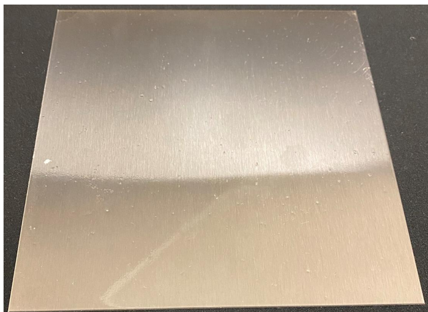
Figure 9. A coupon coated with CLADCO™ provided by FC.
