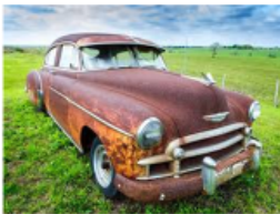
Example of (mostly) uniform corrosion
