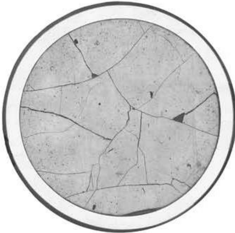
Fig. A.10. Low-magnification cross-sectional photo-composite of Surry Rod H9 at an elevation 510 mm above the fuel axial midplane.
