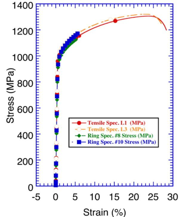
Scaling  $\Gamma$ -Factor calculated using properties of intermediate-strength ferritic steel makes an excellent “blind” prediction of stress-strain behavior of heat treated Inconel 718 ring specimens compared to heat treated Inconel 718 ASTM round bar tensile specimens
