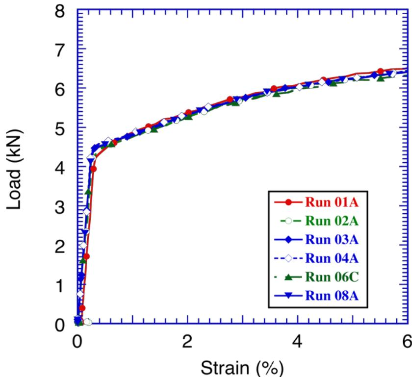
Baseline testing of 6 ferritic steel ring specimens demonstrates consistency of test data obtained using this technique
