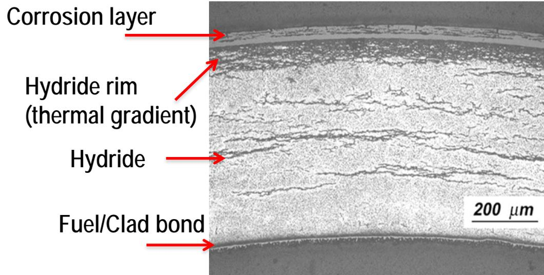
Hydride distribution in as-irradiated high burn-up Zr alloy sample with  $660 \pm 150$  wppm hydrogen.\* Corrosion layer is  $\approx 25 \mu\text{m}$ .
