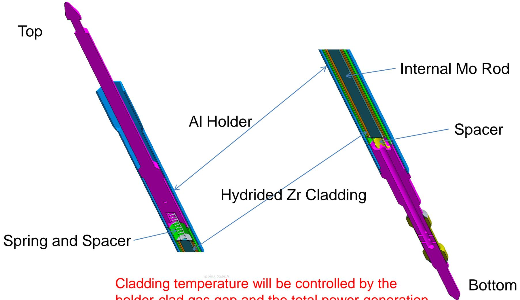
Cladding temperature will be controlled by the holder-clad gas gap and the total power generation within the cladding and the internal Mo rod
