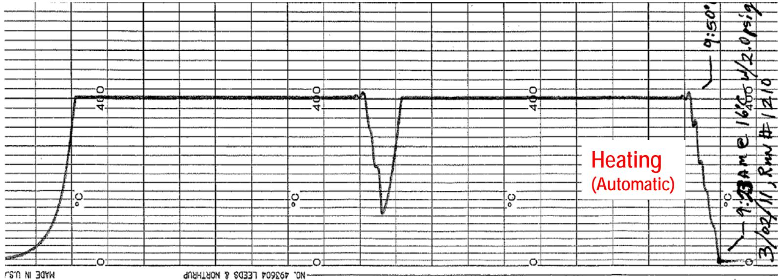
After the samples were initially heated at 400°C for 4 hours, a short thermal cycle (400°C - 120°C - 400°C) was added to obtain uniform hydrogen distribution.
