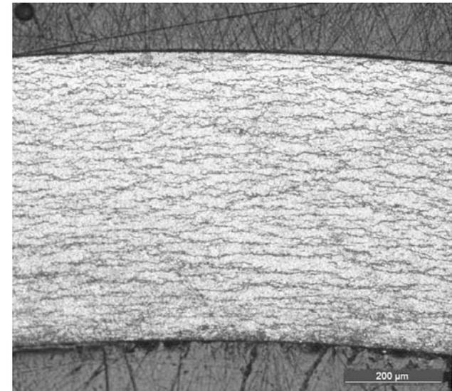
Hydride is uniformly distributed across the cladding wall for an unirradiated two-sided hydrided Zry-4 sample with  $\approx 700$  wppm hydrogen.
