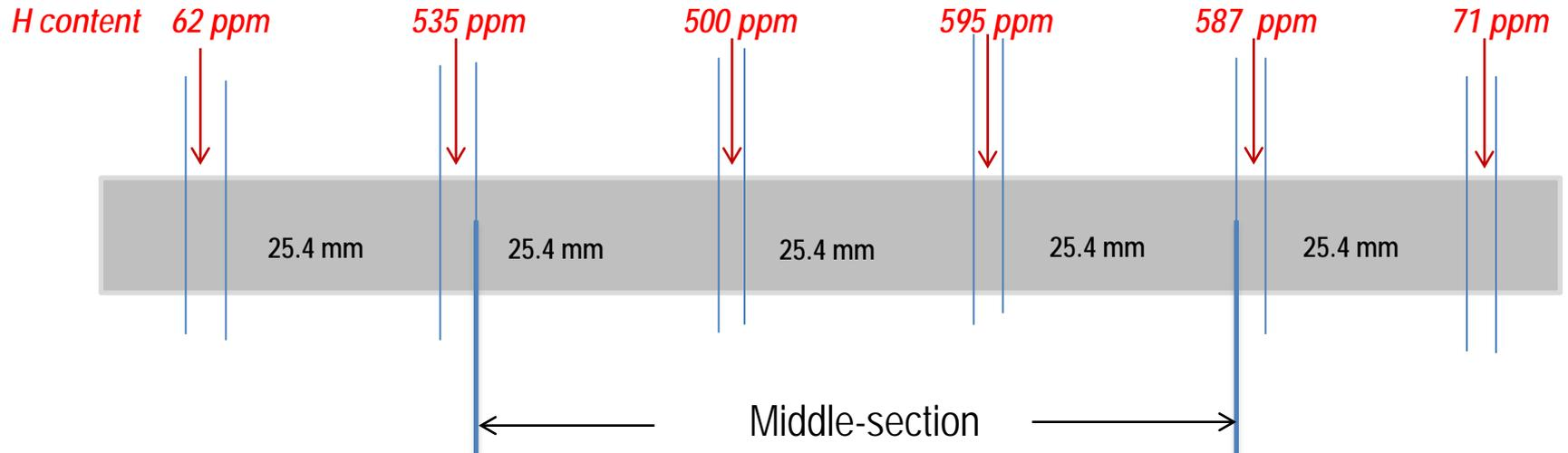
Hydrogen distribution for pre-hydrated Zry-4 sample LRR1D
