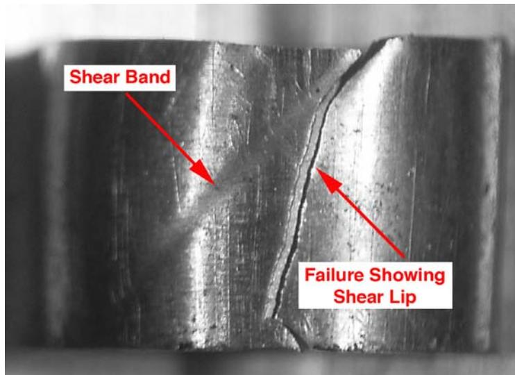
Typical room temperature failure
