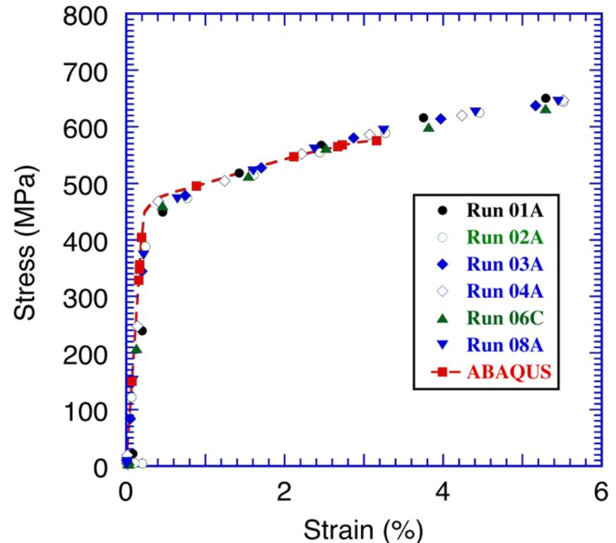
ABAQUS analyses of ferritic specimen using ASTM tensile data as input shows excellent agreement when load data are converted to stress using  $\Gamma$ -factor
