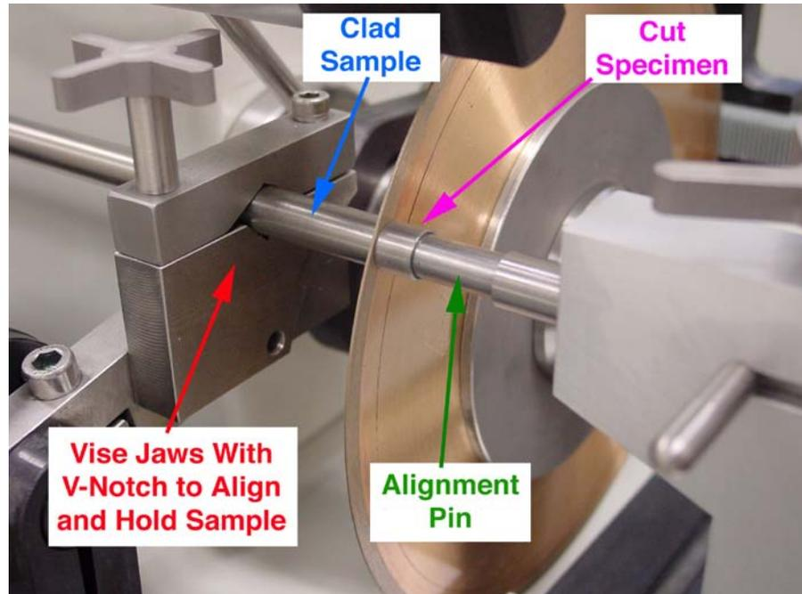
Note: all preparation steps are easily performed remotely in a hot cell environment. Also, there is no specimen machining or modification of outside surface of the specimen.
