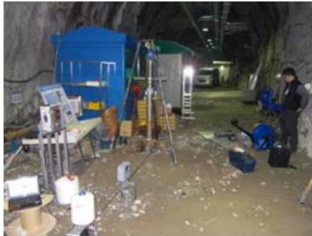
Figure 1. Experimental setup for streaming potential testing
