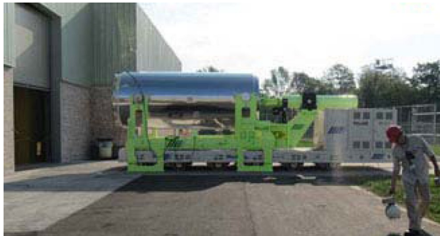
Figure 6-2 SPMT Transporting Horizontal Shielded Cask And Canister From The CRCT Building
