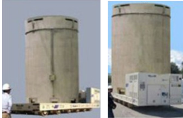
Figure 6-7 SPMT Carrying A UNF Storage Cask
