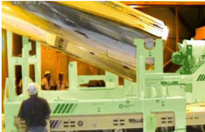
Figure 6-1 Downending a Horizontal Shielded Cask on an SPMT for transfer to the Storage Pad
