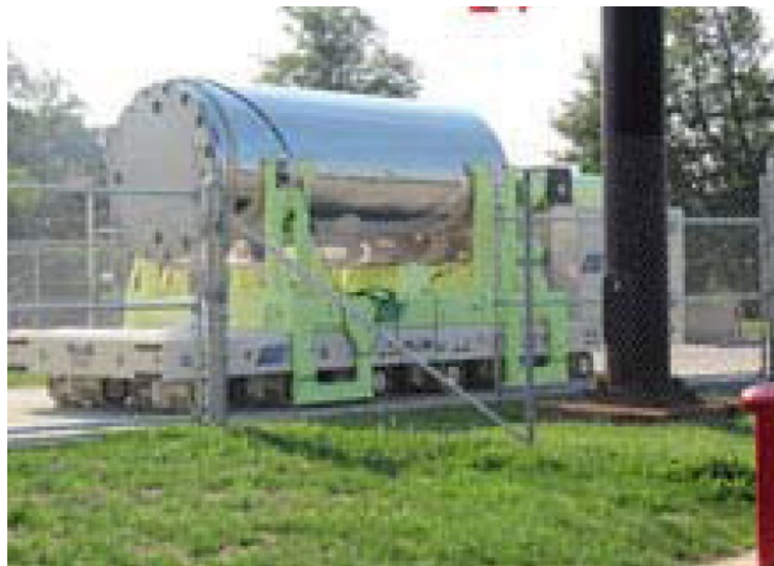
Figure 6-3 SPMT In Transit with Horizontal Shielded Cask and Canister
