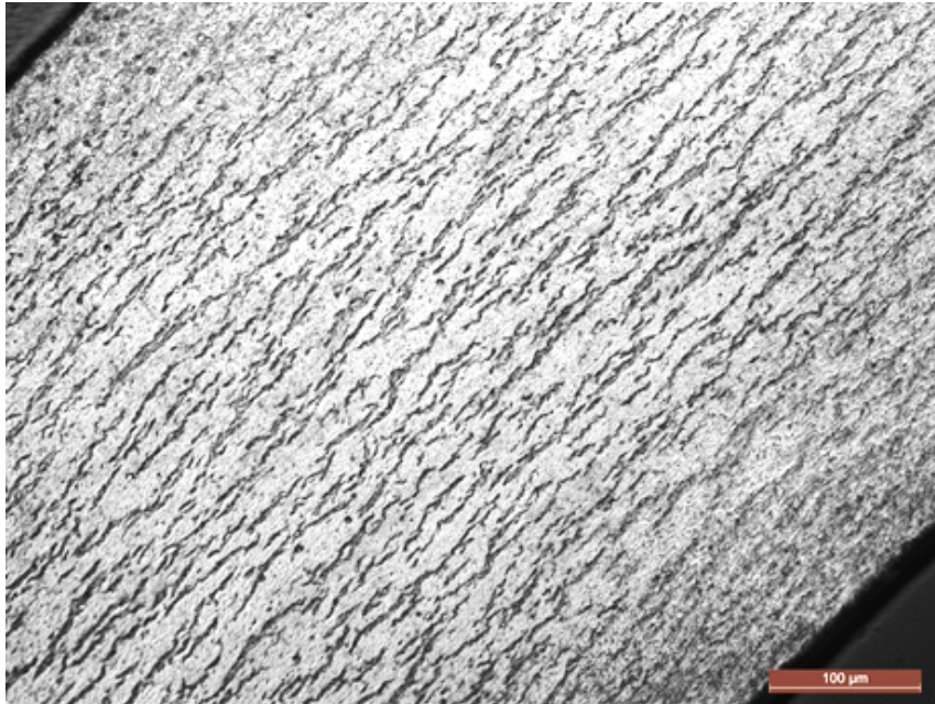
Fig. 2.10. Micrographs showing hydride distributions in hydrogen charged Zircaloy-4 of this study. The average hydrogen contents of this location is \approx 610 wppm.
