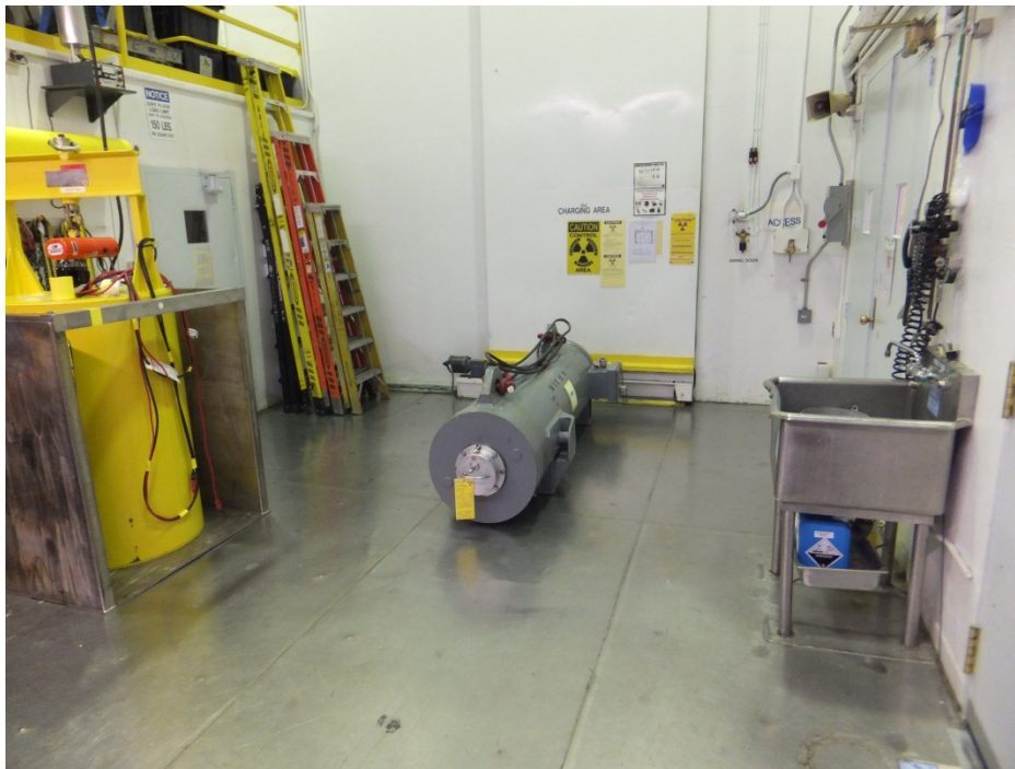
Fig. 4.1. Loop cask for HYCD-1 and HYCD-2 (OD \times L = 2 ft \times 8 ft), at the IFEL.
