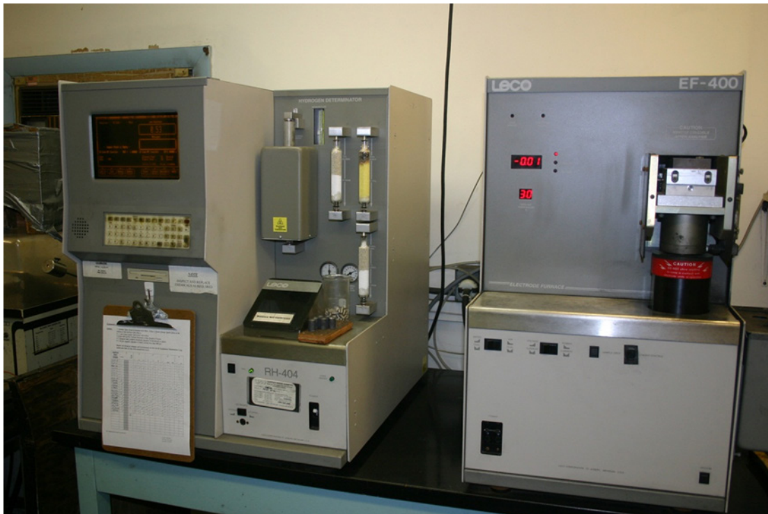
Fig. 2.5. LECO RH-404 Hydrogen Analyzer used for determining the hydrogen content.
