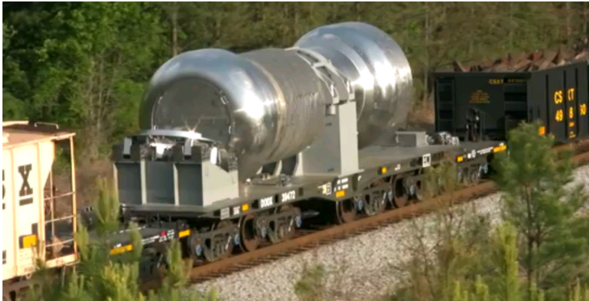
Figure 2.1. Naval UNF Transporter M-290-0001 Cask Car (Meets AAR S-2043)
