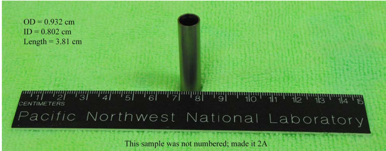
Figure D.3. Photograph of Zr-4 Tube Specimen 2A (vertical orientation)
