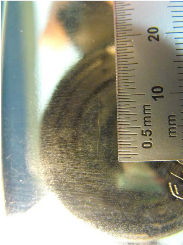
Figure A.12. Crack Specimen 07-343. Gross measurements taken with Vernier calipers.
