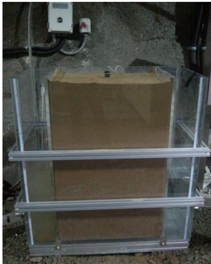
Figure 3-11: Sand box for the preliminary tracer test
