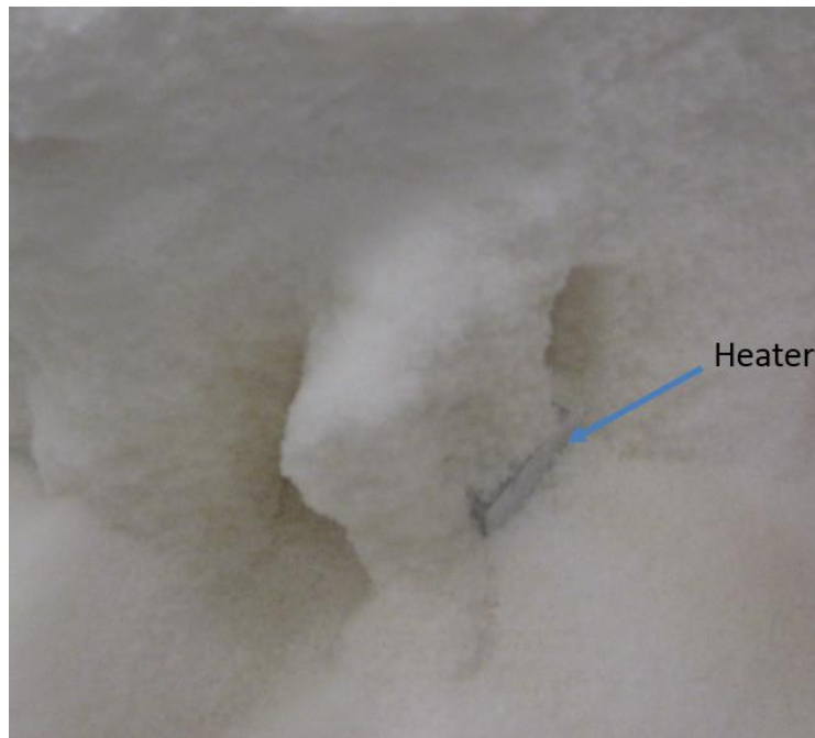
Figure 22. Discolored region around the heater. Some very slight consolidation was observed, as well as some looseness of the salt immediately surrounding the heater. The loose region was significantly firmer and smaller than in Experiment 0 (Figure 20).
