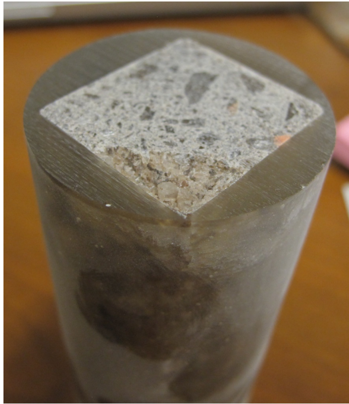
Figure 1: Prismatic reconsolidated salt sample encased in an epoxy coating.
