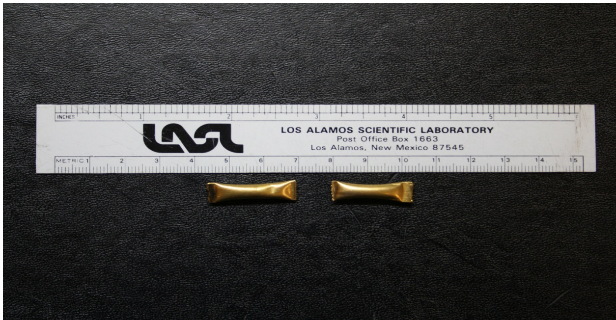
Figure 7) Cold seal system gold reaction capsules, approximately 2.5 cm in length.
