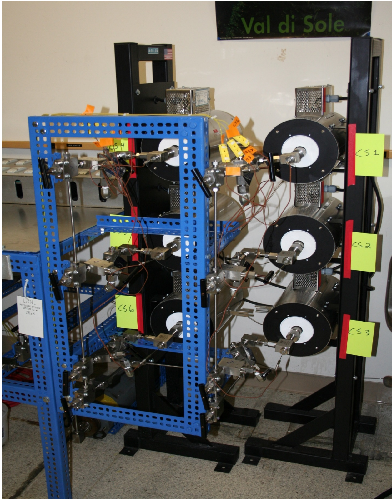
Figure 5) Cold Seal reaction system. Upper temperature /pressure limits are 800 °C, and 2.5 Kb.
