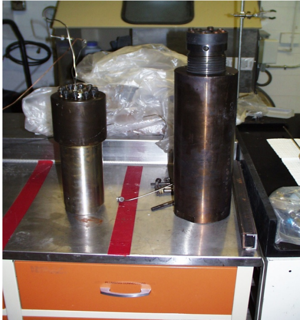
Figure 4) Left: HIP (thrust ring seal type) pressure vessel, for 400c/600bar furnaces Right: AE (bridgeman seal type) pressure vessel, for 600c/1.5kBar furnaces (vessel is ~24" tall)
