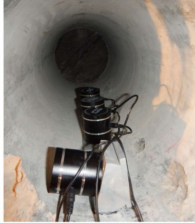
Acoustic Sources in Borehole
