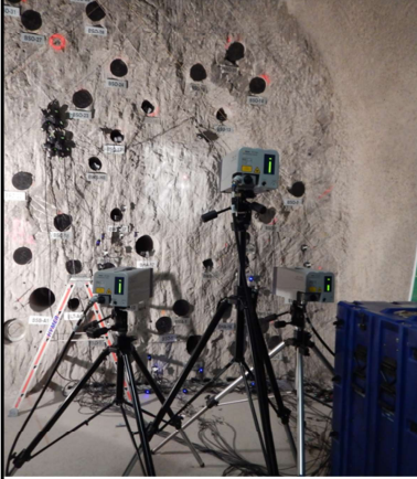
3D Laser Vibrometer in TT-Niche
