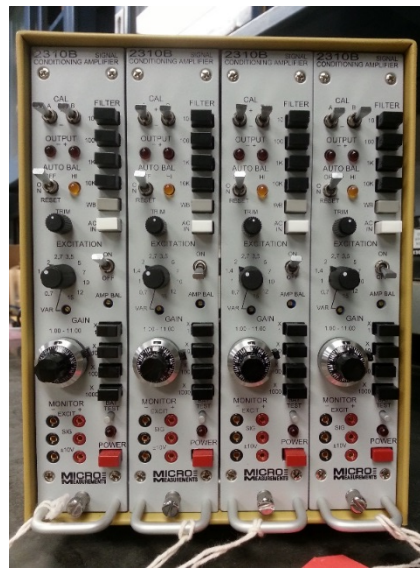
Fig. 6. Strain gage signal conditioning amplifier 2310B, Micro-Measurements.
