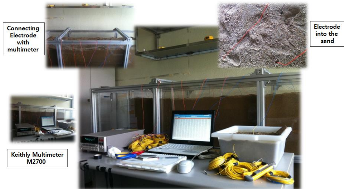
Figure 3: Full set up of a sandbox experiment
