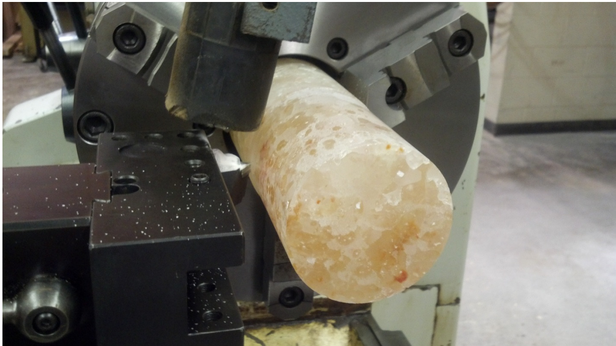
Figure 2. Typical Horizontal Lathe Machining Setup for Preparing Cylindrical Specimens.
