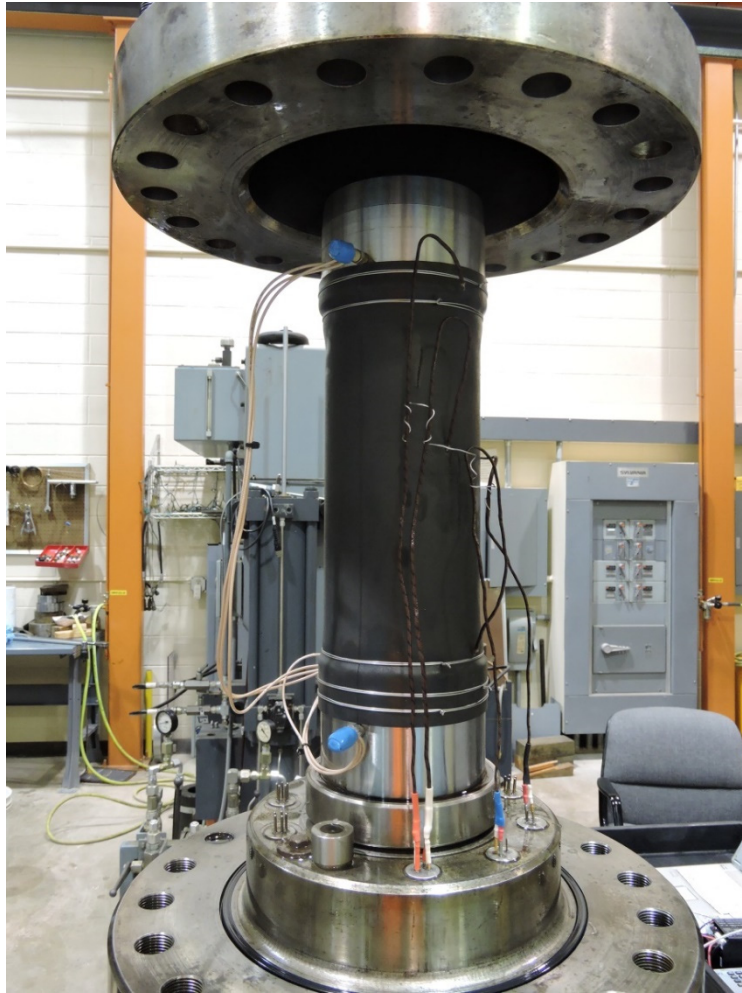
Figure 3. Jacketed Test Specimen in the UTS2 Load Frame With Thermocouples and Acoustic Transducers.
