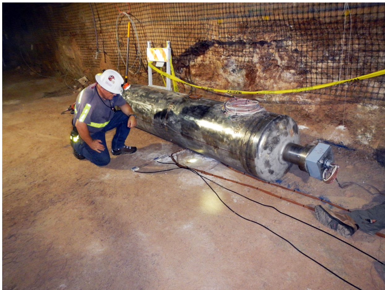
Figure 3: External view of complete canister assembly, placed on drift floor of WIPP prior to addition of RoM salt pile.
