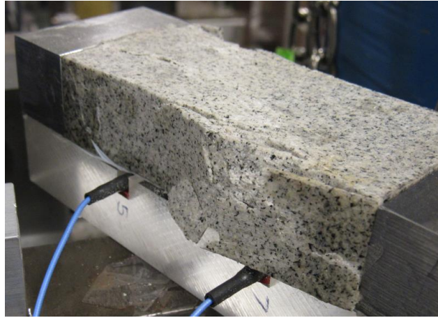
Figure 3-11. Side view of axial-splitting and buckling failure in Sample Z-3.
