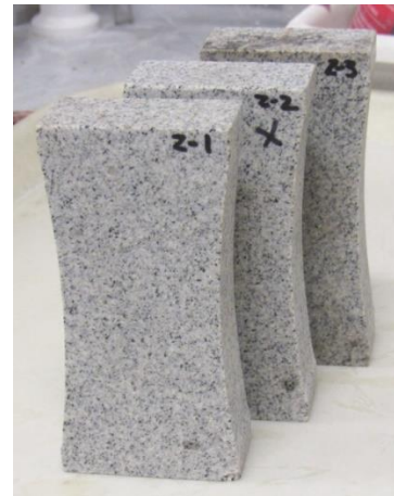
Figure 3-3. Photograph of shaped Westerly granite slabs used for the experiment.
