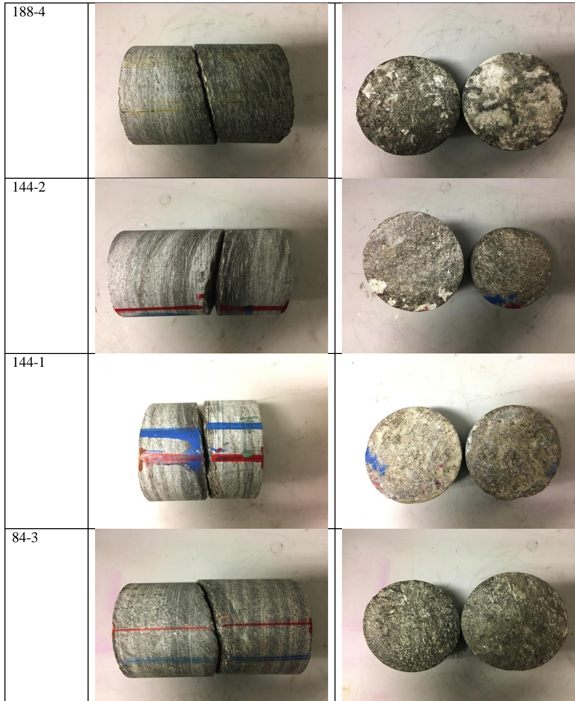
Core samples are 60 mm in diameter. White material seen on core faces 211-2 and 209-3 is sealing material introduced to core during fracture flow experiments and not natural mineralization. White material seen on core faces 188-4 and 144-4 is mineralization (see Table 5-3).
