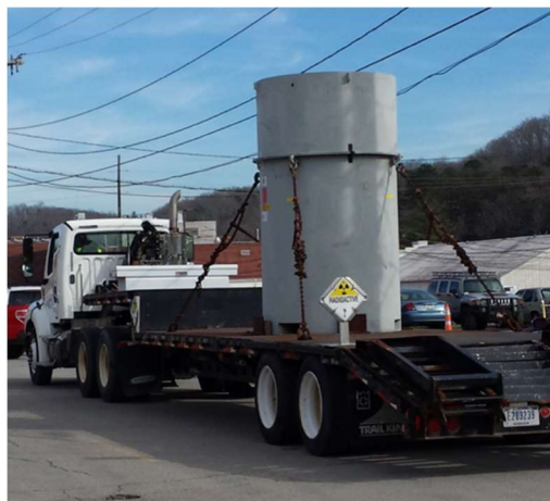
Figure 1. The PWR SNF rods that were loaded into canisters and shipped to TWPC. Image by Bruce Balkcom Bevard.
