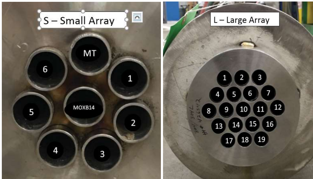
Figure 3. Small and large arrays for storing full length SNF rods in Building 3525 hot cells.
