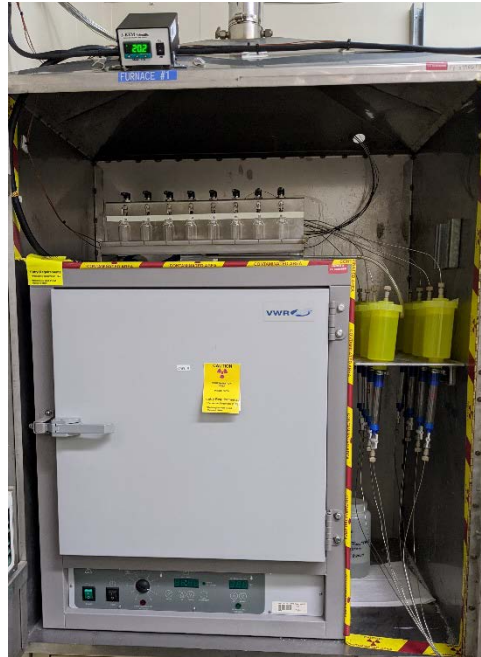
Figure 4.2 The ventilated canopy housing the oven, effluent taps, and funnels directing leachate to ion exchange columns before proceeding to waste.
