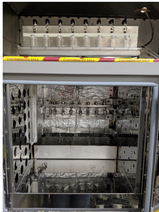
Figure 4.3 Flow cells within the oven in a ventilated canopy.
