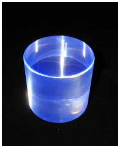
Figure 2. Example of a plastic scintillator under UV light (used with permission from Eljen Technology) [16].
