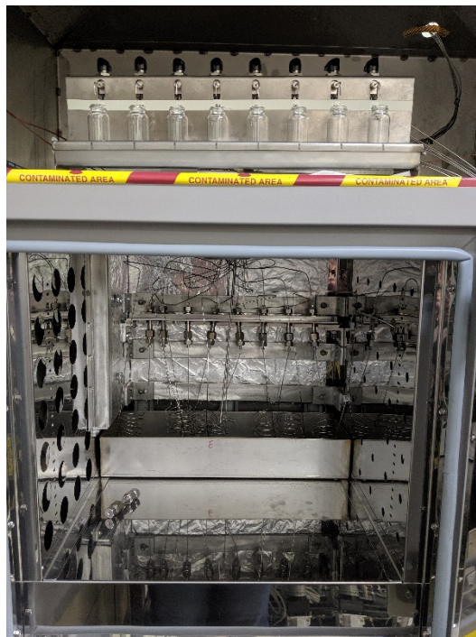
Figure 6. Flow cells within the oven in a ventilated canopy.
