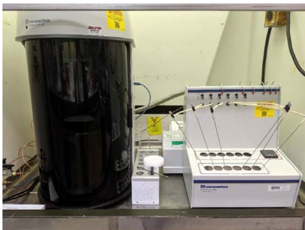
Figure 3. Micromeritics Tristar II Plus analyzer for Brunauer-Emmett-Teller (BET) measurements.
