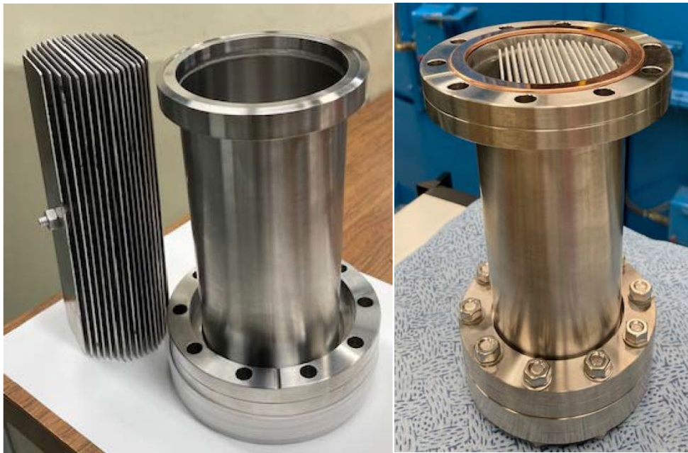
Figure 5-2. Photos of aluminum coupon assembly and corresponding mini-canister from [McNamara and Verst, 2020b]. The proposed sample design will be similar for the oxidized unalloyed Zr material, but axially shortened to accommodate thermal insulation around the mini-canister. Oxidized ZIRLO tubes would be used in a separate mini-canister.
