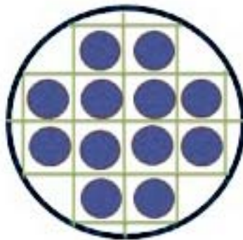
Figure A-11. Option 3a, 12 STAD Handling Frame Configuration
