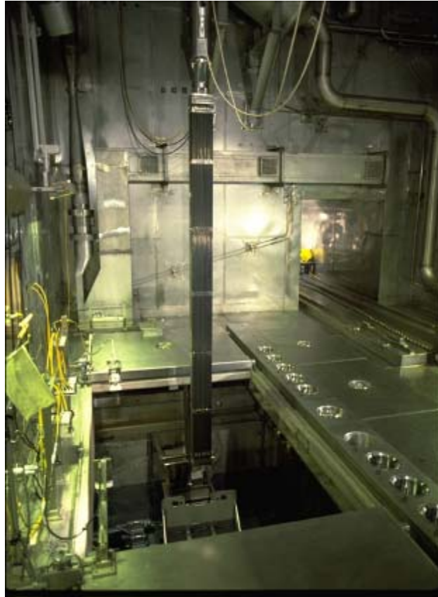
Figure 8-18. Repackaging the UNF from the Transport Canister into a New Configuration at the T(0) Facility
