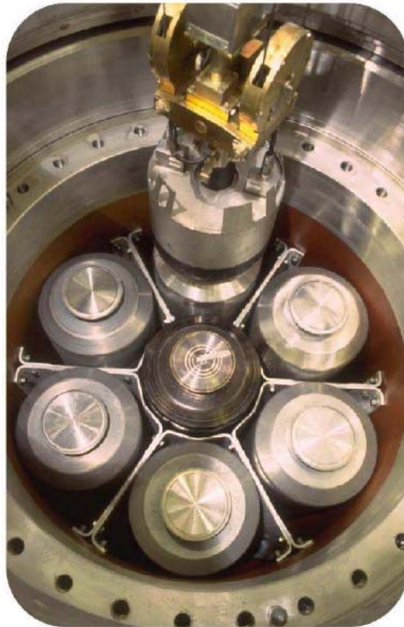
Figure 8-4. 12 High Level Waste Overpack for Transportation
