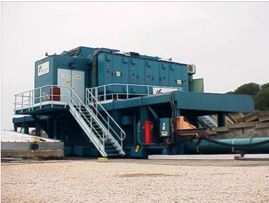
Figure 8-12. Example of Mobile Hot Cell Used to Repackage HLW in Europe
