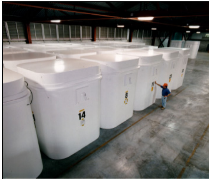
Figure 4.4 DSC Storage at Pickering
